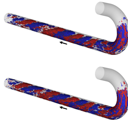
Figure 4: Isosurfaces of the velocity component normal to the equatorial plane ( u_y ) of (top) POD mode 17 and (bottom) POD mode 18 for 180°-bend with laminar inflow. Red surfaces indicate positive values, whereas blue surfaces represent negative ones. The black arrow indicates the flow direction.
